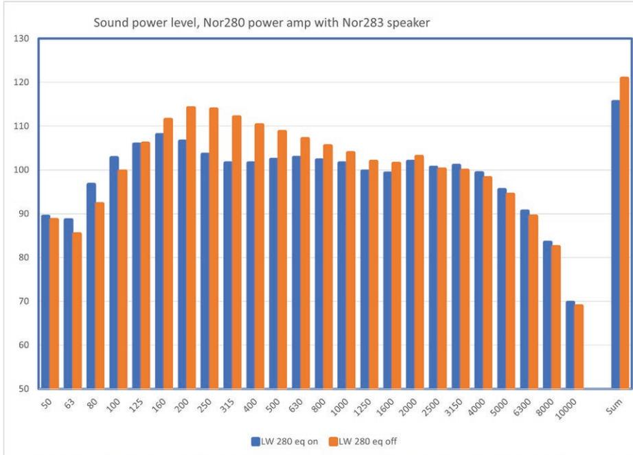
Typical sound power level vs. frequency of the loudspeaker Nor283 when used with the pink noise source and equalizer included in the power amplifier Nor280.
