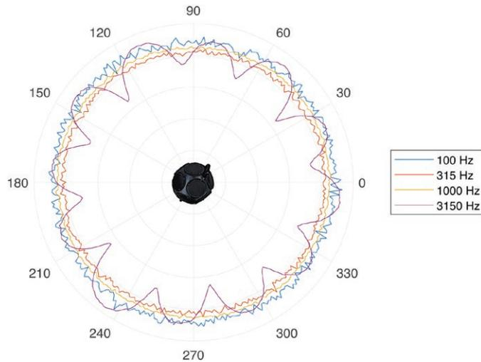
Sound power in different directions for Nor283. The measurement is done in a horizontal plane through the centre of the loudspeaker for the frequencies 100 Hz, 315 Hz, 1 kHz and 3,15 kHz. Each concentric circumference represents a difference of 10 dB with its adjacent ones.
