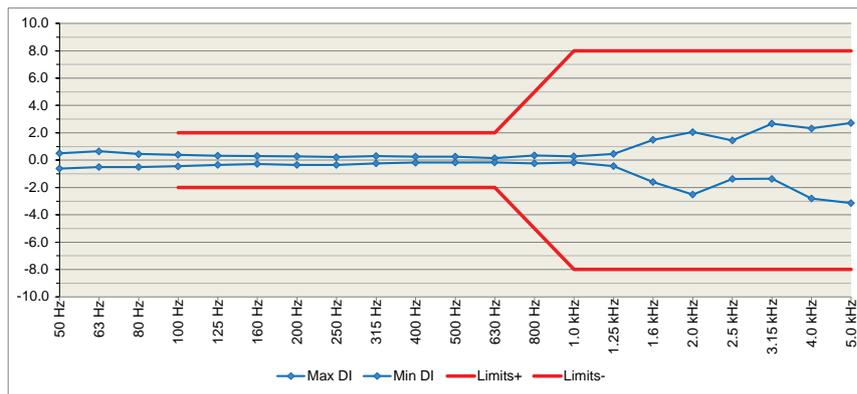
Maximum and minimum directivity indices in different directions according to the requirements in ISO 10140-2:2021 and ISO 16283-1:2014 compared to the tolerance limits.
