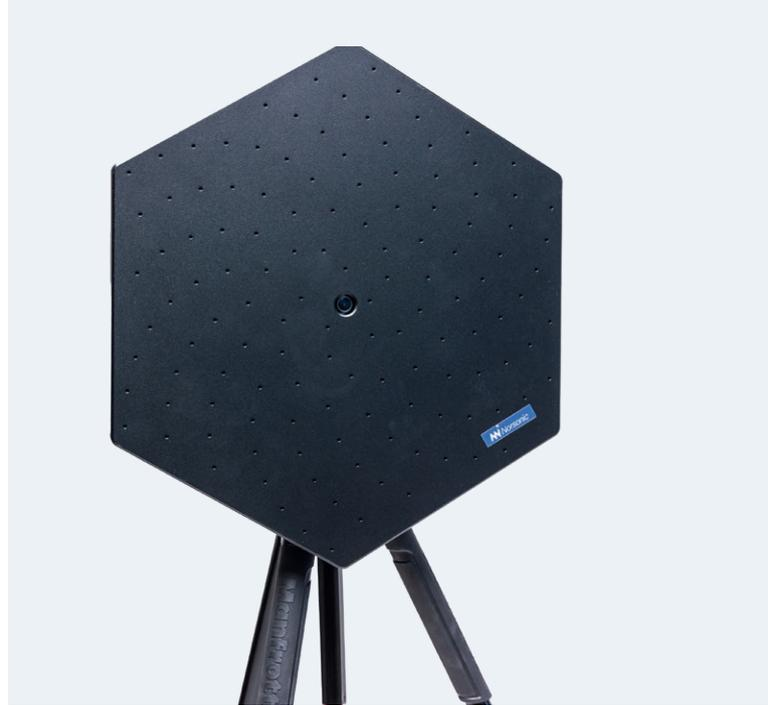
The Hextile is a robust and lightweight aluminium construction, has 128 MEMS microphones, and is less than 3 kg in weight while having a maximum diameter of 46 cm.
