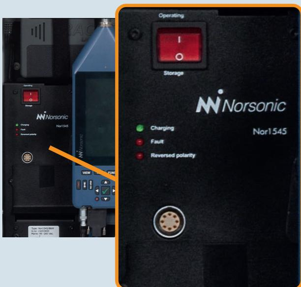
Figure 3: Status LEDs and Operating switch
