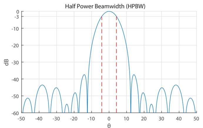
Fig. 2. Two-sided opening angle for half power beamwidth.
