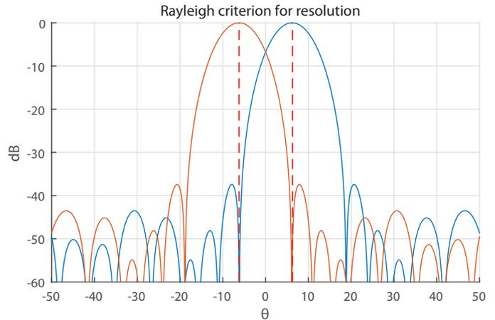
Fig. 1. Rayleigh criterion for resolution of two waves of equal strength and equal frequency. The mainlobe peak of the beampattern for one wave falls on the first zero of the beampattern of the other.
