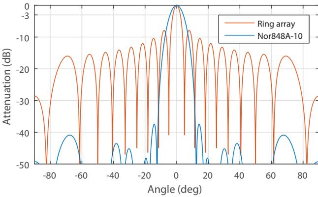
Fig. 19. Beampattern of Nor848A-10 and ring array with same number of elements and same diameter simulated at 3 kHz.
