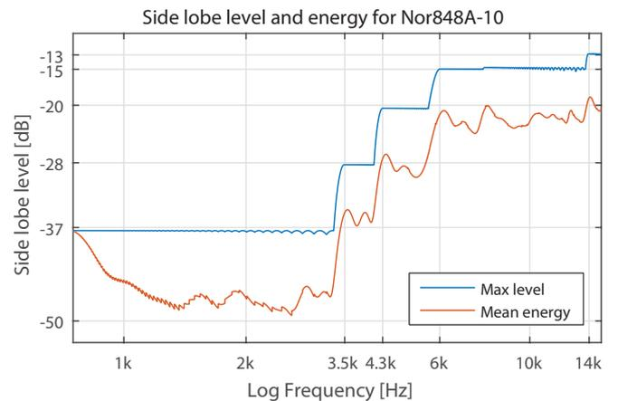
Fig. 17. Maximum side lobe level and mean side lobe energy as a function of frequency for the Nor848A-10 acoustic camera
