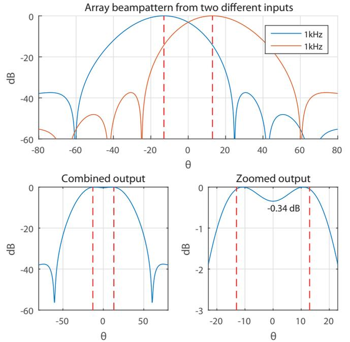
Fig. 7. Two equally strong incoherent sources at 1 kHz placed  $25.4^\circ$  apart. Bottom left shows the overall output of the array when the input consists of both sources, with bottom right displaying a zoomed in view.
