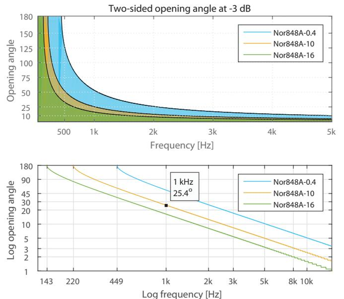
Fig. 5. Two-sided opening angle (HPBW) as a function of frequency for three different array sizes. The two-sided opening angle at 1 kHz is marked for the Nor848-10 at  $25.4^\circ$ . On the bottom part of the figure both opening angle and frequency is plotted in logarithmic scale.
