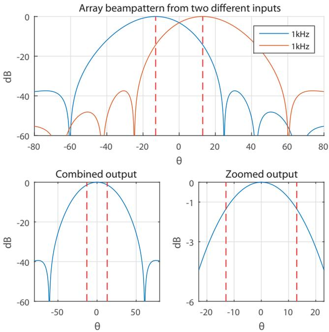
Fig. 11. Two equally strong coherent sources at 1 kHz placed 25.4° apart. Bottom left shows the overall received beampattern from both sources, with bottom right displaying a zoomed in view.
