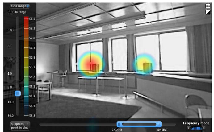
Fig. 13. Resolution of two loudspeakers with white noise output by using Nor848A-10 1.0m camera
